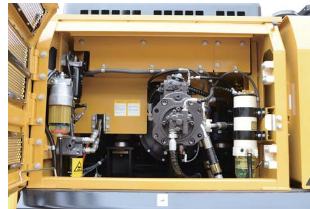
Large-capacity multi-stage filter system
